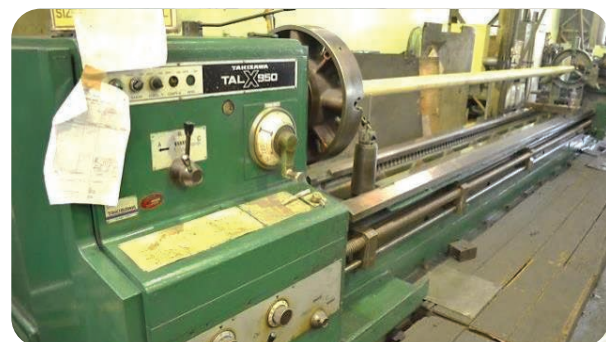
Lathe Machine (Max. Capacity Ø 950 mm x L 10,000 mm)
