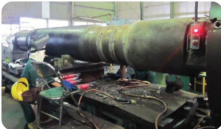
Lathe Machine (Max. Capacity Ø 1,200 mm x L 10,000 mm)
