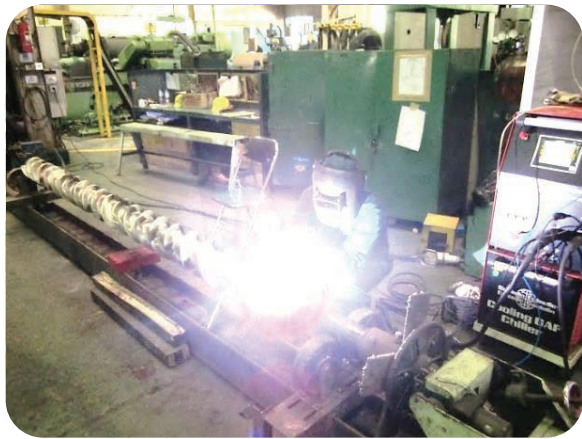
Plasma Transferred Arc Welding on Injection Screw
