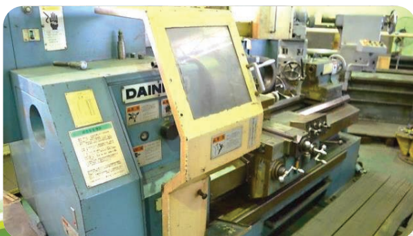
NC Lathe Machine (Max. Capacity Ø 500 mm x L 1,000 mm)
