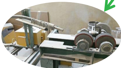
Shot-blaster Machine and the mechanical rotation is controlled fully from the outside of the room.
