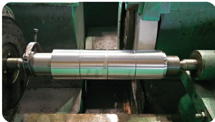
Supporter Cylinders [Ø 150 mm x 110 L mm]
