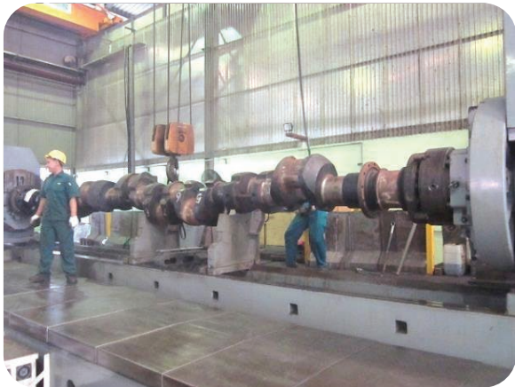
8,500 mm Crankshaft Grinding Process on CNC
