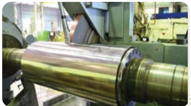
Calender Roll for Rubber [Ø 462 x SL 1,020 x TL 2,760 mm]
