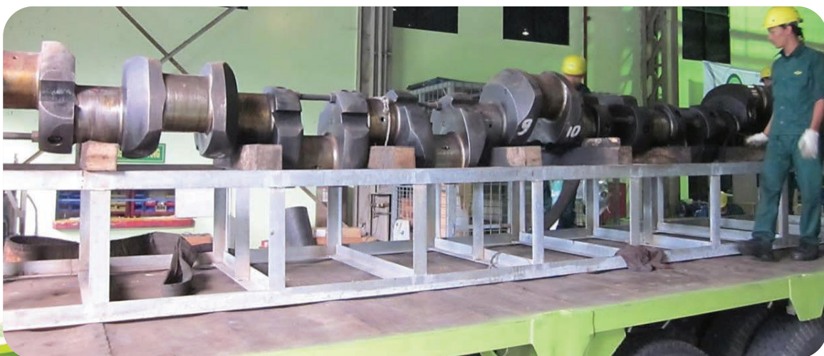
Overhaul of Crankshaft 7,000 mm in Length
