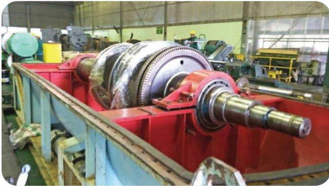
Steam Turbine Rotor 20 MW [Ø 406 x TL 5064 mm]
