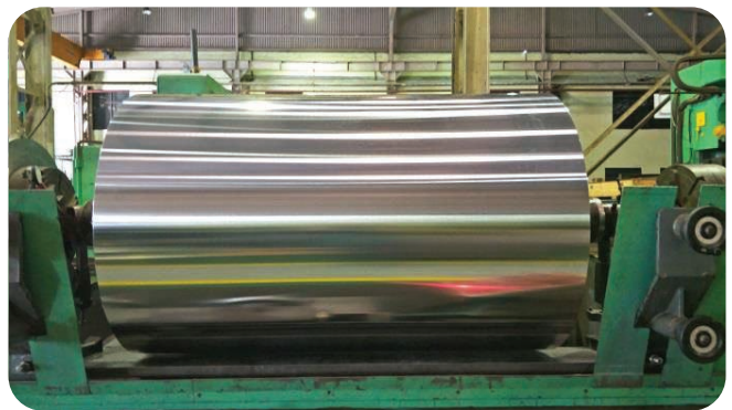
Cooling Roll Finishing Grinding [Ø 900 x TL 1500 mm]
