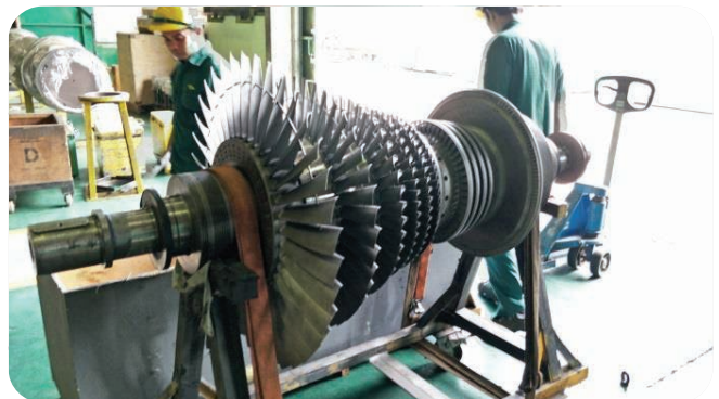
Rotor Turbine [HVOF Coating Finishing Grinding]
