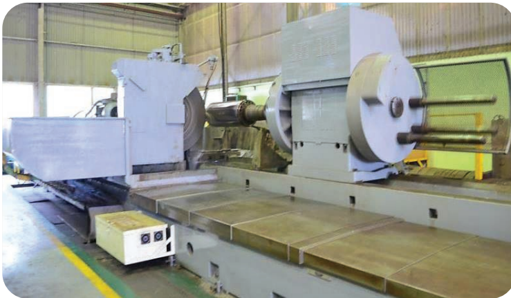
CNC Cylindrical Grinding Machine (Max. Capacity Ø 1,600 mm x L 8,500 mm)
